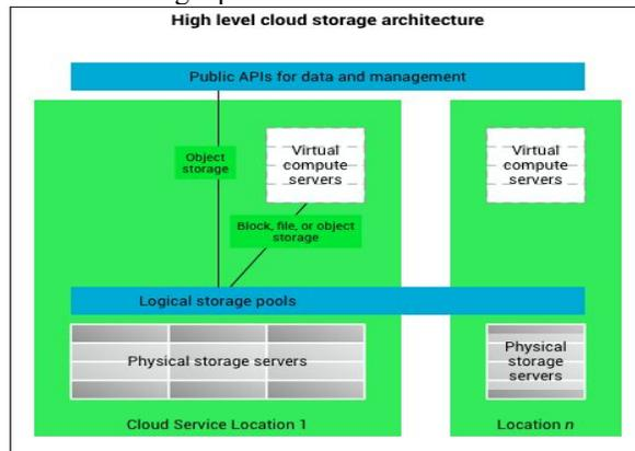
Figure 1. Architecture of data sharing in cloud storage.
