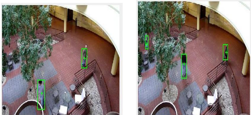
**Fig 7. Objects tracked from video based on result obtained from Pattern Classification-based Adaptive Background Update Method**
