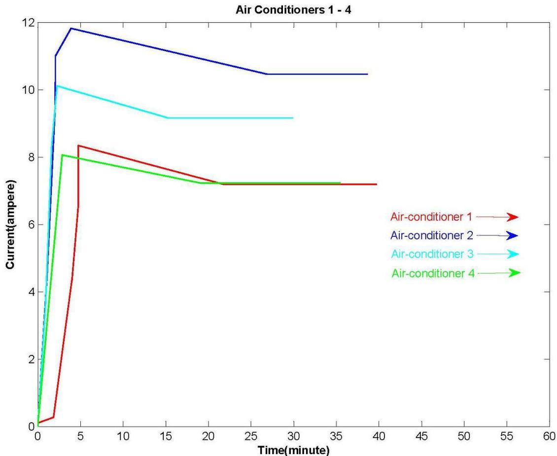
Fig [2] – Current and Time graph of air-conditioners in cold load pickup condition
