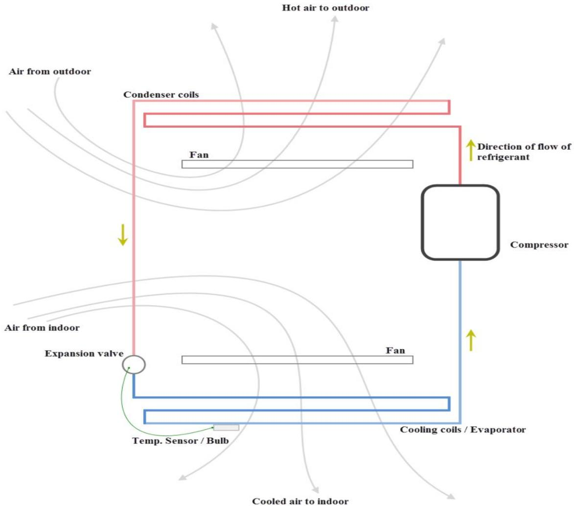
*Fig [1] – Simple Air conditioner mechanism*
