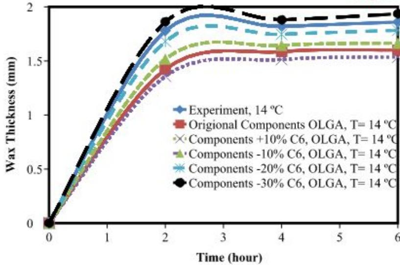
Figure 9: The effect on the predicted wax thickness of changing crude oil components, using OLGA at a flow rate of 2.7 L/min and an inlet coolant temperature of 14°C.
