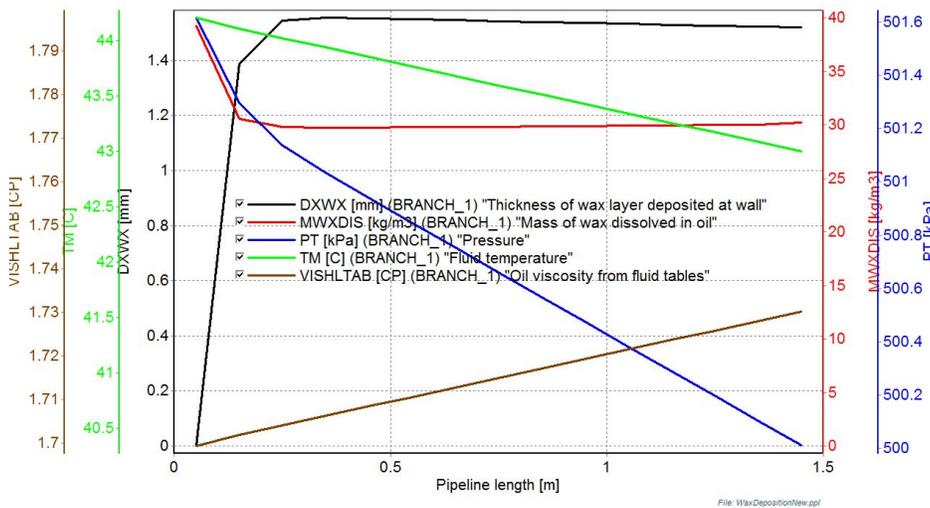
Figure 6: Simulation output of wax deposition profile along the test section pipe of the experimental rig for this study, at a flow rate of 4.8 L/min.
