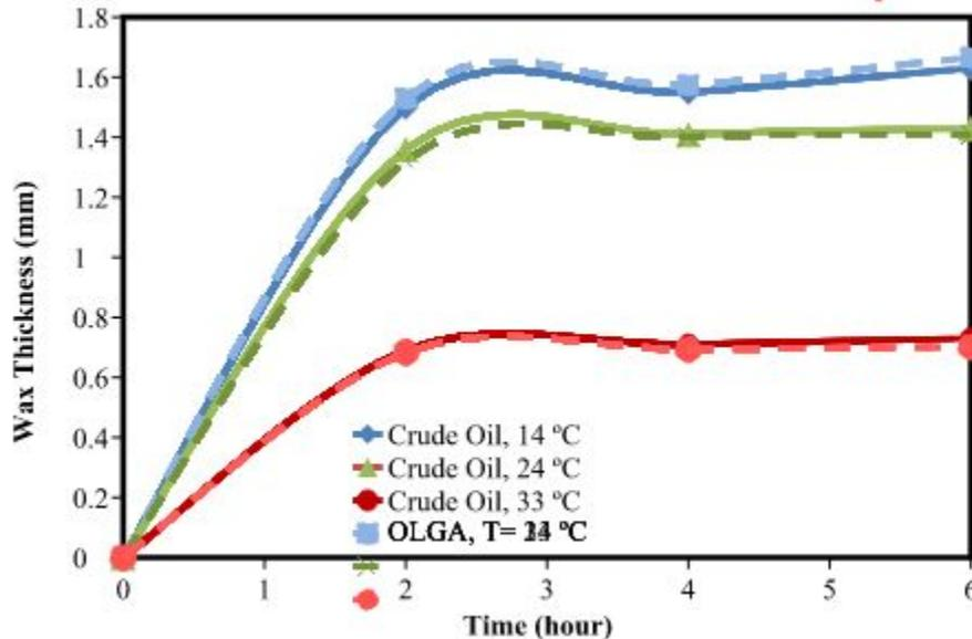
Figure 12: Comparison between the experimental results and the simulation results at a flow rate of 4.8 L/min.
