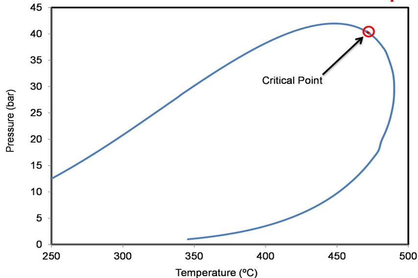
Figure 4: Phase envelope of the crude oil used for wax simulations using PIPESim.
