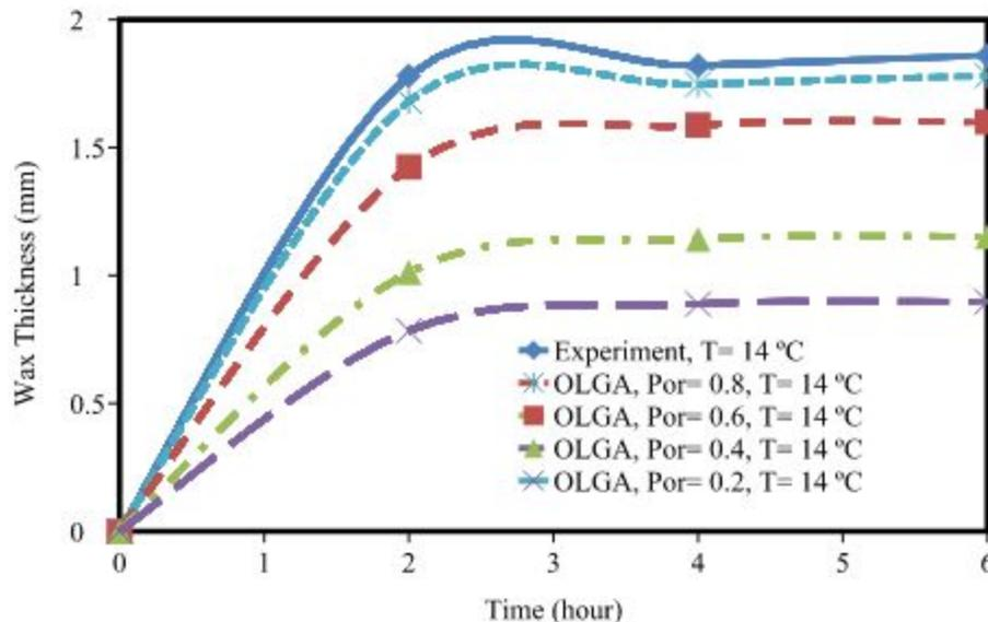
Figure 7: The effect of wax porosity on predicted wax thickness at flow rate 2.7 L/min and an inlet coolant temperature of 14°C.
