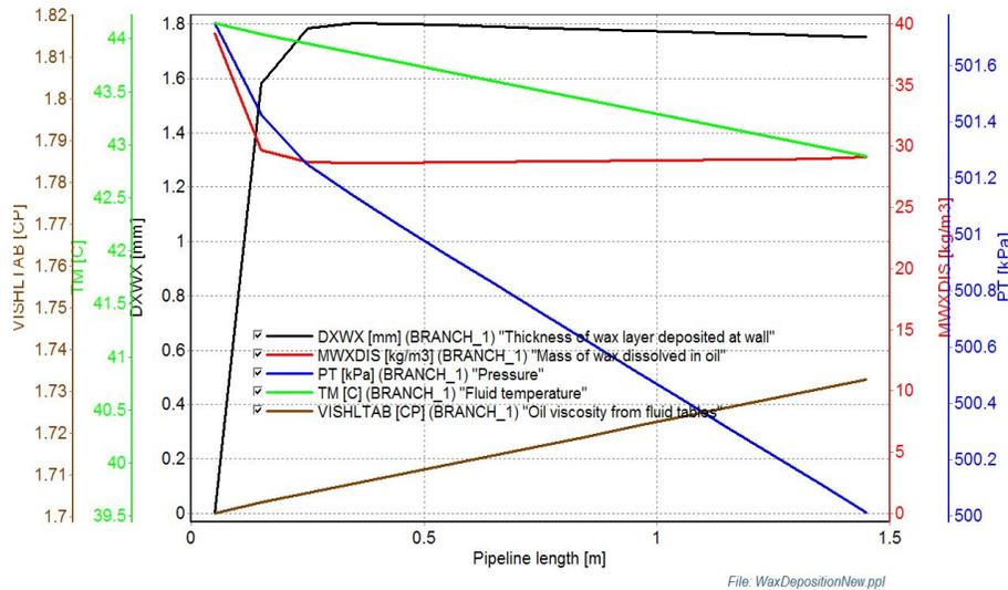
Figure 5: Simulation output of wax deposition profile along the test section pipe of the experimental rig for this study, at a flow rate of 2.7 L/min.
