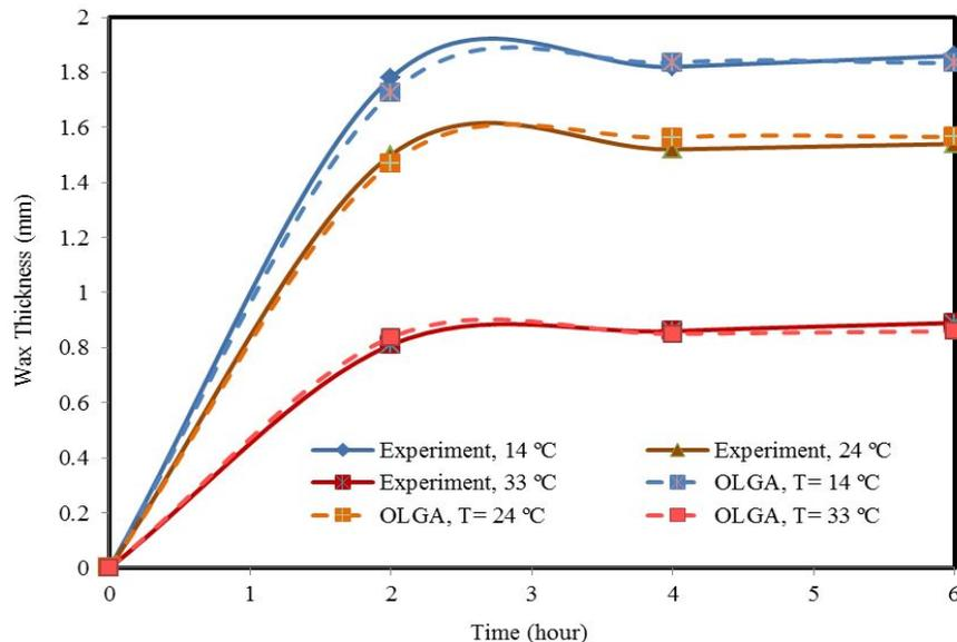
Figure 11: Comparison between the experimental results and the simulation results at flow rate 2.7 L/min.
