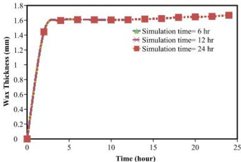
Figure 10: The effect of simulation time on the wax thickness at 2.7 L/min, an inlet coolant temperature of 14°C and a wax porosity of 0.6.
