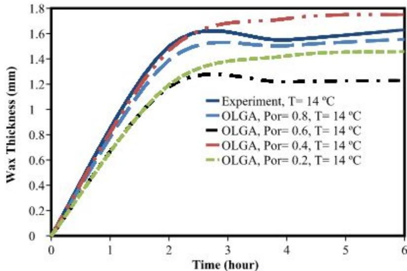
Figure 8: The effect of changes in wax porosity in OLGA simulation on predicted wax thickness at flow rate 4.8 L/min and an inlet coolant temperature of 14°C.
