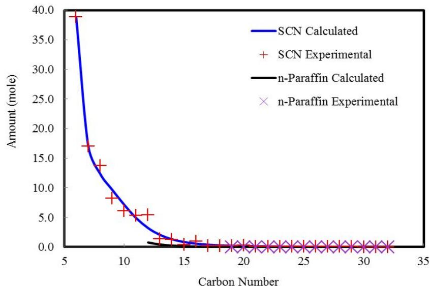
Figure 3: Distribution of the single carbon number (SCN) in the crude oil and the n-Paraffin using PIPESim.
