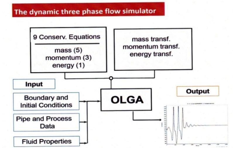
Figure 1: Steps of the OLGA simulation process [5].
