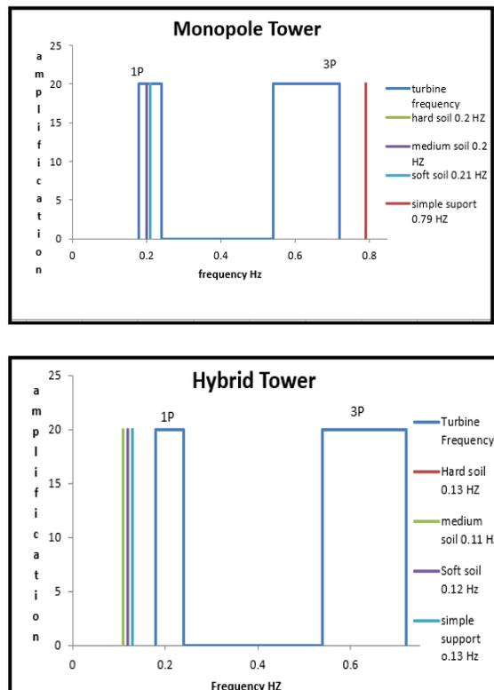
Fig. 3. Comparison of frequency in monopole and hybrid tower for different soil conditions
