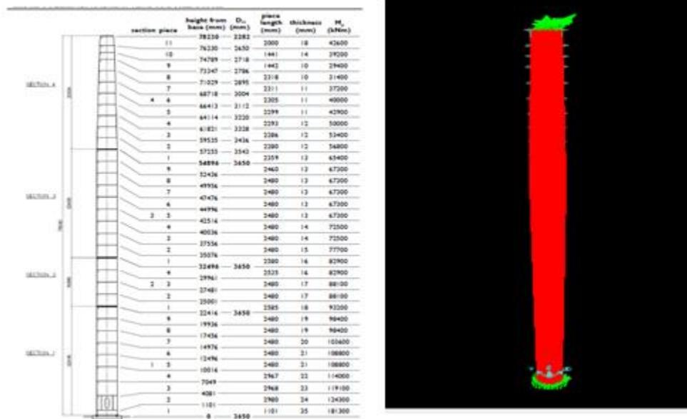
Fig. 1. Details Of 78-meter-high tower and its FEM model
