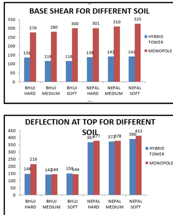
Fig. 4. Comparison of base shear and displacement for monopole and hybrid tower in different soil conditions
