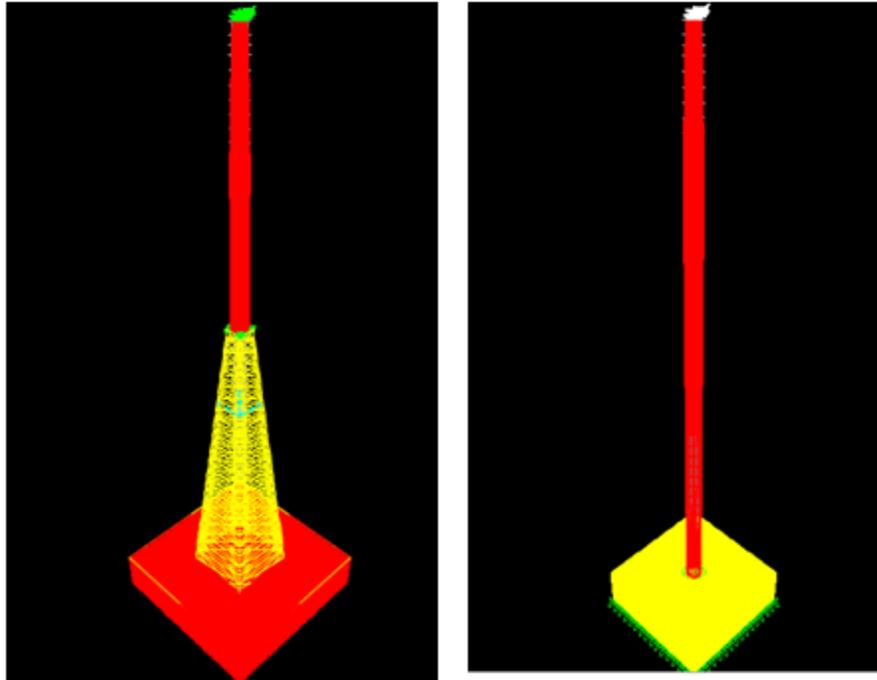
*Fig. 2. FEM model of 125-meter-high monopole and hybrid tower with soil*
