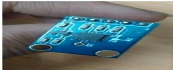
*Fig 3. MEMS Accelerometer*
