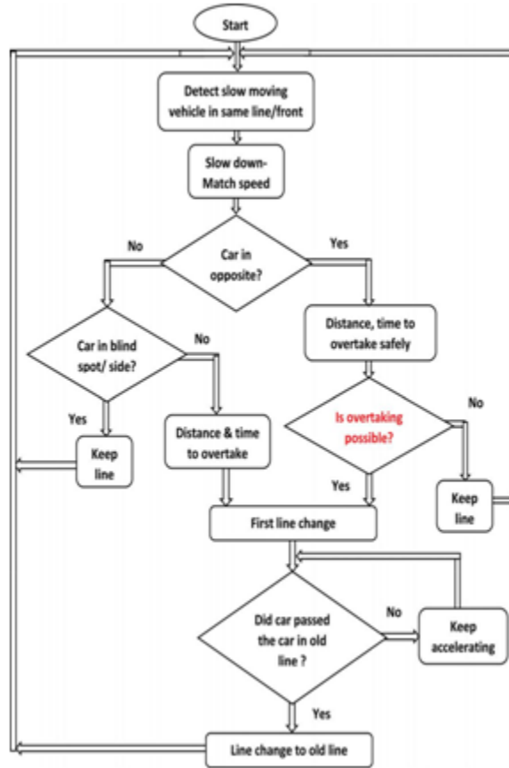
Fig. 6: Overtaking assistance - Collision warning algorithm
