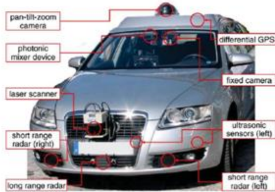
Fig. 3: A vehicle with Advanced Driver Assistance Systems
